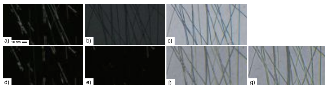
Figure 6.16: Empty PVP fibres with reflecting parts. Upper row: original appearance at room temperature viewed through crossed polarisers in reflection (a) and transmission (b) and without polarisers in transmission (c). Lower row: sample on heating at 95°C (d), 105°C (e,f) and 110°C (g).
