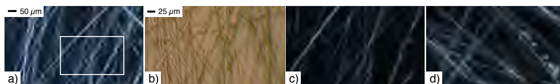
Figure 7.3: Composite fibres with the LC elastomer as core and PVP as sheath observed through crossed polarisers (a) and without them (b). Note that (b – d) show the marked area in the larger magnification. On rotating the sample from (c) to (d) the birefringence of the core is visible with its director along the fibre formation axis.
