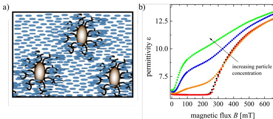
Figure 1: a) Scheme of LC polymer brush particle, b) Capacitance measurements with parallel  $B$  and  $E$  field for pure 5CB (black) and 5CB doped with a) 9OCB-PHMS@CoFe<sub>2</sub>O<sub>4</sub> and in volume fractions from 0.01 vol% up to 0.1 vol%..
