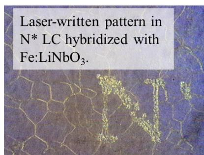
Figure 1: Pattern in a N\* LC sample (no doping, no dyes), written with a scanned laser beam.
