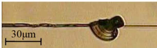
Figure 1: "Seashell" structure formed along a liquid crystal fiber diluted with velocity \geq 7.1\mu\text{m/s} [2].
