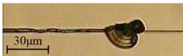
Figure 2: "Seashell" structure formed along a liquid crystal fiber dilated with velocity \geq 7.1 \mu\text{m/s} [2].
