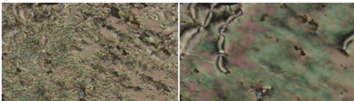
Figure 1: Planar textures of a studied nanocomposite: a) without UV-light, b) under UV-light.
