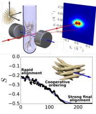
Figure 1. Experimental SAXS setup and evolution of order parameter over time showing cooperative ordering of a CNC chiral nematic suspension.
